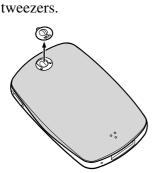
2 Slide the back over of the player down, and then lift up, as shown by the arrow below.
